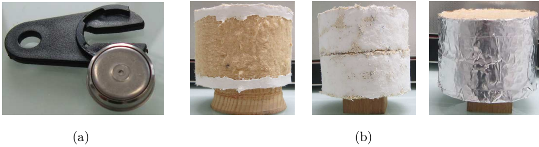
Figure 3. Sensors of relative humidity and temperature (a) and wood fibre samples (b) with white acrylic seal and with aluminium tape.
