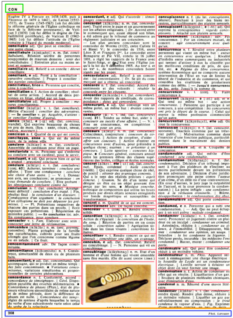
Fig. 1: First and second segmentation levels of a dictionary page
