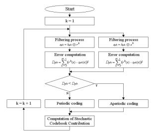
Figure 3.2 : Flowchart of the PMF-CELP coding
