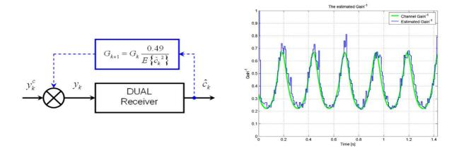
Fig. 7. a) Block diagram for the statistical gain control loop; b) Estimated G parameter and the inverse channel gain
