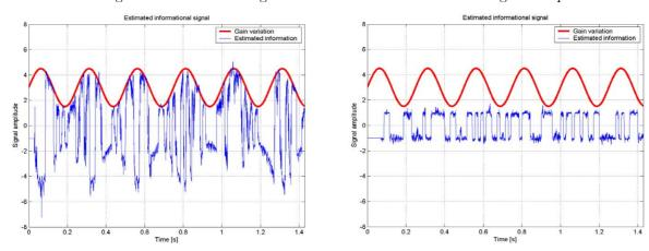
Fig. 5. Estimated information and channel gain for: a) modified system model; b) adaptive statistic loop
