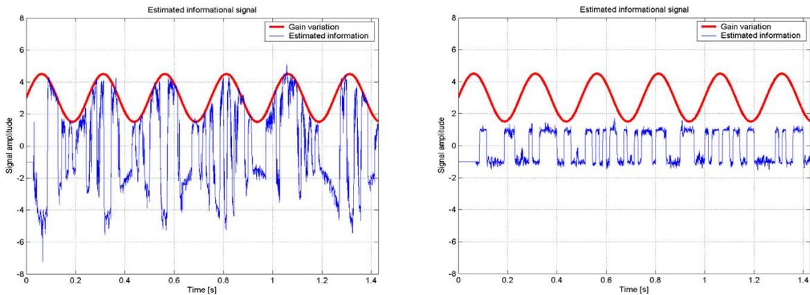
Fig. 5. Estimated information and channel gain for: a) modified system model; b) adaptive statistic loop
