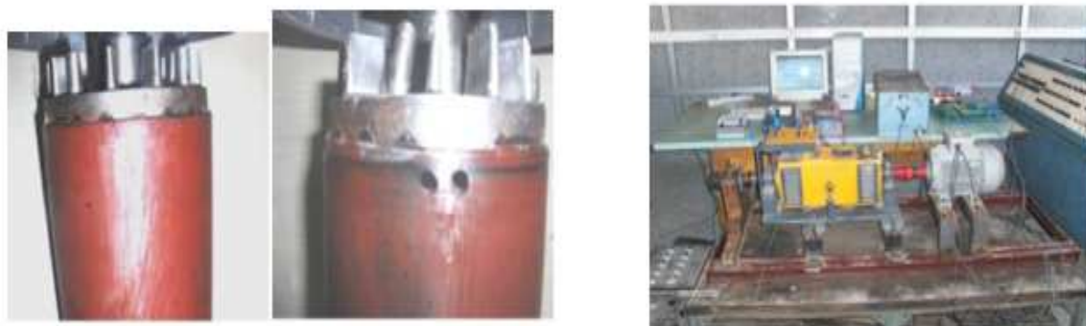
Figure 1: From left to right, healthy rotor and 2 Broken Bars, snapshot of the experimental test Bench
