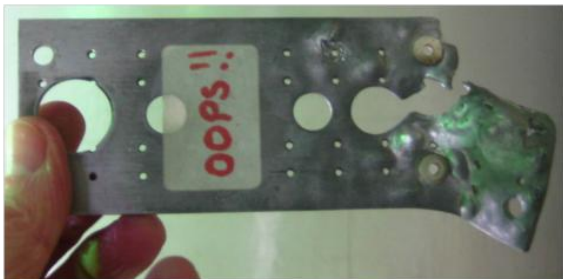
Figure 18: Ion Beam Damage. Energy deposition effects of a high power beam (200 keV, 0.2 mA)
