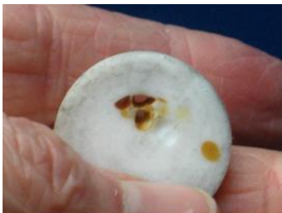
Figure 19: Enhanced electronic sputtering of insulators. PTFE disc, 5mm thick. Irradiated with \sim 1 MeV protons in \sim 1993-4 to do machine calibration using the resonant \text{F}(p, \gamma) reaction at 990 keV for work reported in (Kazor et al. 1994)
