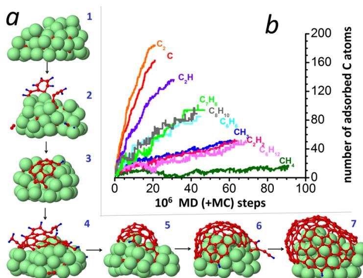
**Figure 6** (a) Nucleation process of a CNT from  $C_nH_m$  species on a Ni nanocatalyst, which is physisorbed on a virtual Al or Si substrate. Here, Ni, C and H atoms are in green, red and blue colors, respectively; (b) evolution of adsorbed C atoms on/in the Ni nanocluster during the CNT nucleation from different hydrocarbon species. For the sake of clarity, the different cases are presented in different colors.
