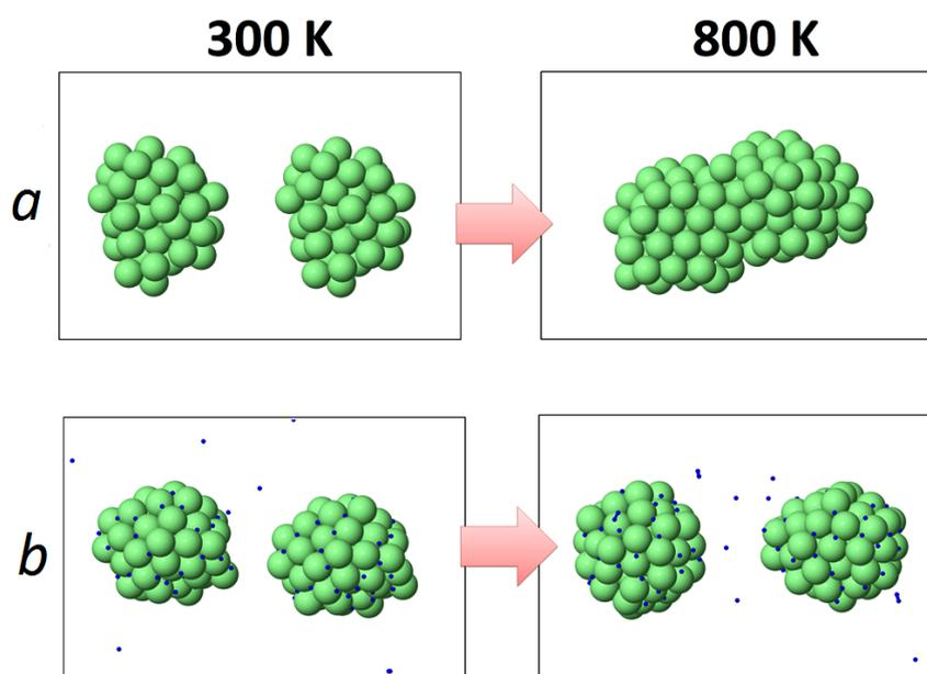
**Figure 5** Top views of the interaction of two  $\text{Ni}_{55}$  nanoparticles on a virtual Si surface at temperatures of 300 K and 800 K in the regimes of annealing, (a) without and (b) with  $\text{H}_2$ -plasma. Here, Ni and H atoms are shown in green and blue colors, respectively.
