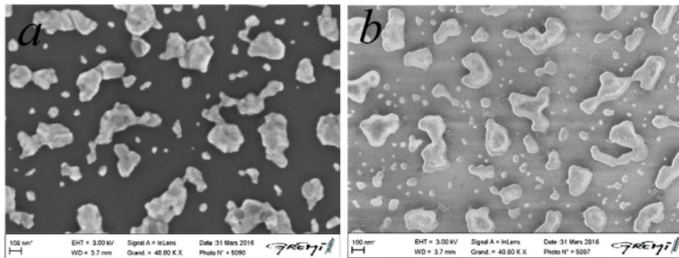
**Figure 4** SEM images after the annealing of Ni film (white) with initial thickness of 6 nm on Si/SiO<sub>2</sub> substrate (black) at 650°C, (a) without and (b) with applying a H<sub>2</sub>-plasma.
