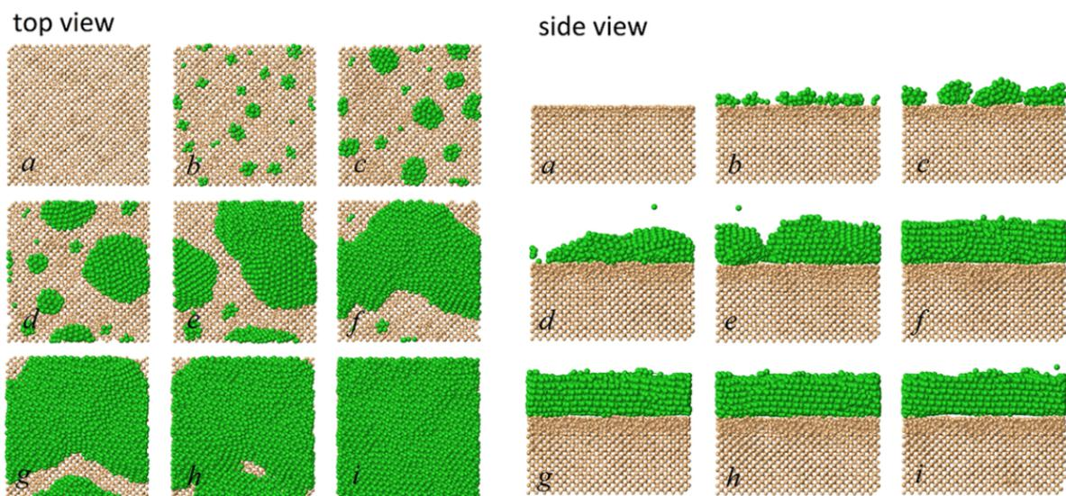
**Figure 1** Snapshots of top and side views of the simulation cell during deposition of Ni atoms (green) on the Si(100) substrate (brown) at room temperature.
