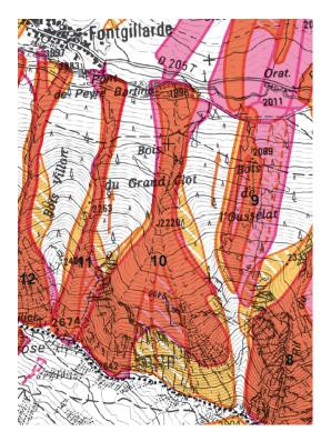
**Figure 3.** The Localization Map of Avalanche Phenomena (CLPA) in Molines-en-Queyras township. The CLPA path number 10 corresponds to the EPA path number 7 presented in Fig. 1. The avalanche extension limits obtained from eyewitness accounts are plotted in magenta. The yellow contours show avalanche extension limits based on photo-interpretations. Orange areas represent the intersection of these two contours.
