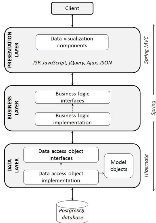
**Figure 7.** Architecture of the web application for entry and management of avalanche observations.
