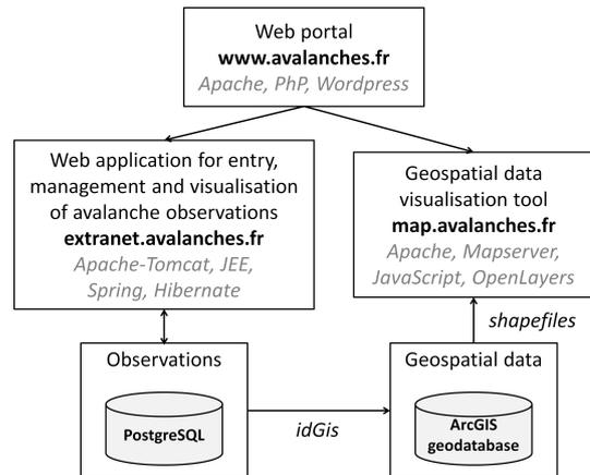
**Figure 6.** Main components of the information system.
