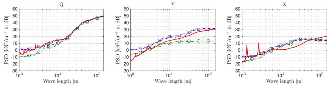
Figure 26. PSD of contact forces, front wheelset in alignment, constant velocity. Experimental data (red line), numerical simulations with track geometry irregularities with KLE error equal to 10% (dotted green line with circle markers), 1% (dashed blue line) and 0.1% (dotted violet line with square markers).
