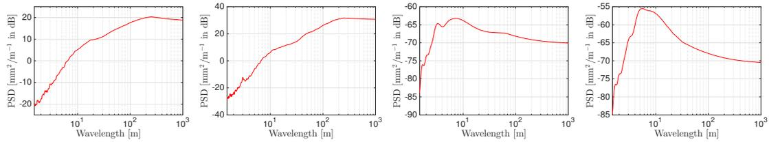
Figure 8. Experimental PSD of geometry irregularities, from left: gauge, superelevation, horizontal curvature and vertical curvature.
