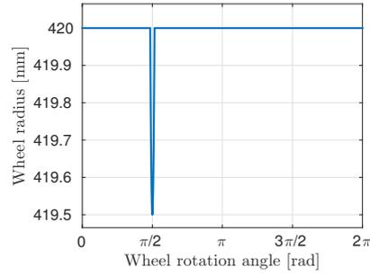
Figure 28. Wheel untrue used for the numerical simulations.
