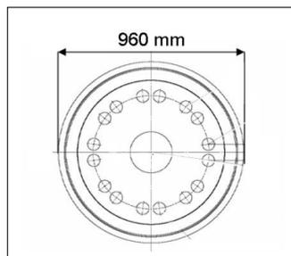
Figure 20. Position of the strain gauges used for the contact forces measurement on a wheel.
