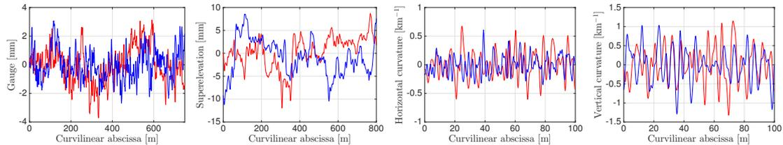
Figure 17. Example of geometry irregularities, from left: gauge, superelevation, horizontal curvature and vertical curvature. Measurements (red line), generations (blue line).
