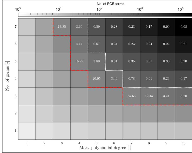
Figure 14. Percentage error in the PCE identification ( $\varepsilon_{PCE}$  in Equation 12) of the vertical curvature irregularity (100 KLE terms). The dashed red line delimits the area in which the identification is not possible since the number of PCE terms is lower than the number of KLE terms to model. The dotted white line delimits the area in which the PCE error is lower than 1%.
