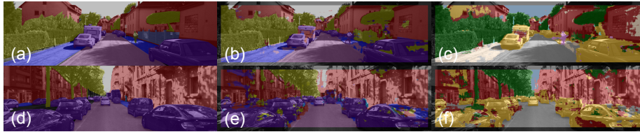
Figure 4: Example of pixel classification results given by the JTSC strategy (see Figure 1). (a) is the ground truth from the Ros et al. labelset. (b) is the result obtained with our strategy for the same labelset and (c) is the result obtained for the Kundu et al. labelset. (d) is a ground truth image from He et al.. (e) is the result obtained with our strategy for the same labelset and (f) is the result obtained for the Xu et al. labelset.
