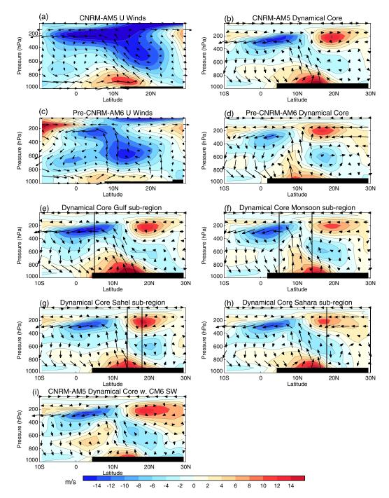
Figure 11. As Figure 7, but for a cross section (10W – 10E) of U winds (colours, ms<sup>-1</sup>), with V winds and Omega shown as vectors, and subregions indicated by vertical black lines.
