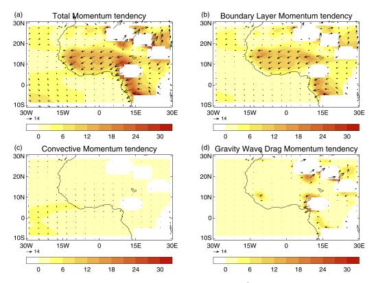
Figure 8. HadGEM2-A August-mean parametrized momentum tendencies at 925 hPa (ms<sup>-1</sup>/day). (a) Total momentum tendency (excluding those from advection), (b) boundary-layer scheme tendency, (c) convection scheme tendency, and (d) Gravity-wave drag scheme tendency. Grid-points where 925hPa is below the surface are masked in white.
