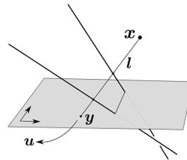
Figure 1. A general camera associates a scene point  $x$  with a visual ray  $l$ , then maps the ray  $l$  to its intersection  $y$  with some retinal plane  $\pi$ , and finally uses a projective coordinate system on  $\pi$  to express  $y$  as a point  $u$  in  $\mathbb{P}^2$ .
