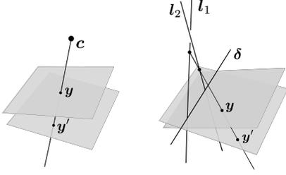
Figure 2. *Left*: A pinhole  $c$  induces a homography between any two retinal planes not containing  $c$ . *Right*: Two skew lines  $l_1, l_2$  induce a homography between planes intersecting at a transversal  $\delta$  to  $l_1, l_2$ .
