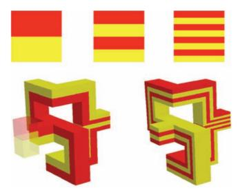
**Fig. 1.** Illustration of a 3D mixing pattern. Top: Cross-section illustrating the Baker's transformation after two iterations. Bottom: sketch of mixing actions after two elements [11].
