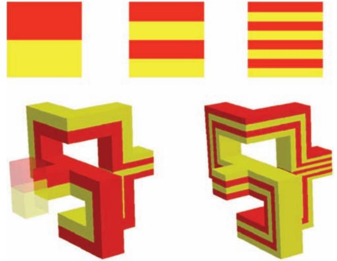
**Fig. 1.** Illustration of a 3D mixing pattern. Top: Cross-section illustrating the Baker's transformation after two iterations. Bottom: sketch of mixing actions after two elements [11].
