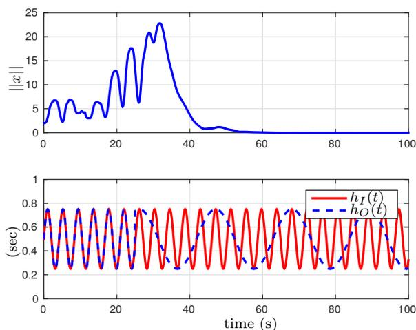
Figure 1. Top: Norm of the state – Bottom: Known Delays  $h_I(t)$  and  $h_o(t)$  used to compute the prediction
