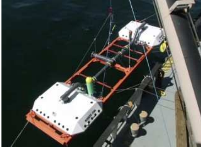
Figure 1: The scale prototype of the M3 WEC during its deployment offshore the coast of Oregon in September 2014.
