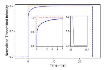
Figure 3: Example of transmitted signal observed in our experiments for a power sent on the ruby crystal of about 1.6 W and a pulse duration  $\tau_{in}=25\,\mathrm{ms}$  (solid line). The dashed line is the profile of the incident pulse obtained by replacing the ruby crystal by a suitable neutral density filter. The insets are enlargements of the pulse rise and fall.
