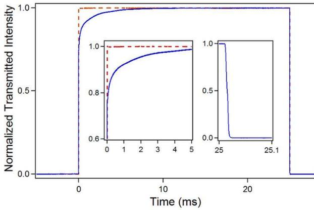
Figure 3: Example of transmitted signal observed in our experiments for a power sent on the ruby crystal of about 1.6 W and a pulse duration  $\tau_{in} = 25$  ms (solid line). The dashed line is the profile of the incident pulse obtained by replacing the ruby crystal by a suitable neutral density filter. The insets are enlargements of the pulse rise and fall.
