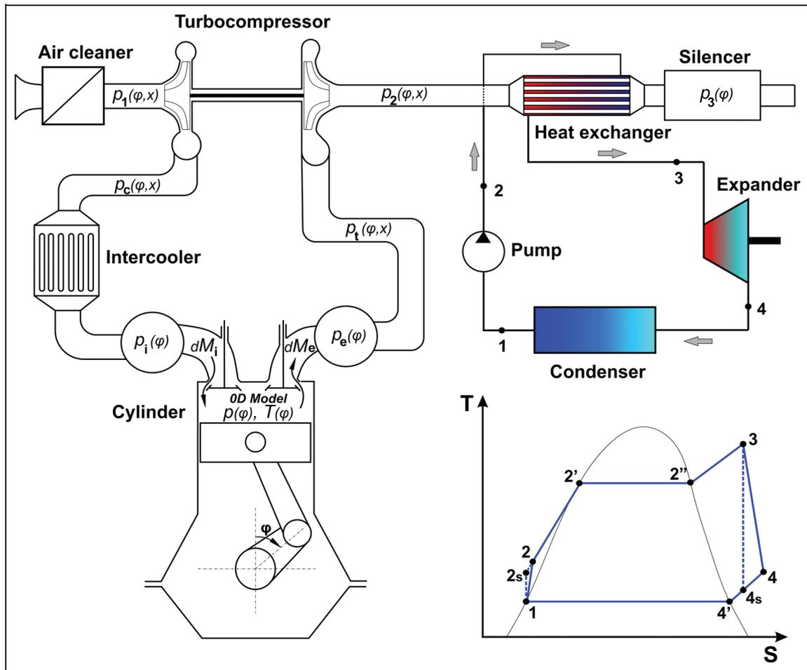
**Figure 1.** Models of the engine and the RC.
