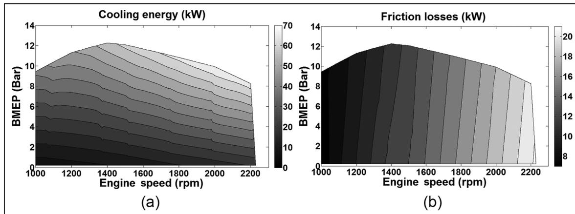
**Figure 4.** (a) Waste heat through the cooling system; (b) friction losses.
