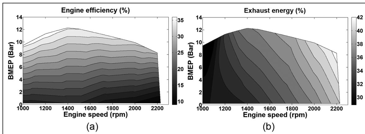
**Figure 5.** (a) Engine efficiency; (b) exhaust energy.
