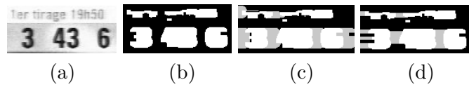
Figure 4: Original image (a) binarized accumulated gradients (b) after conditional dilation (c) and after conditional erosion (d).
