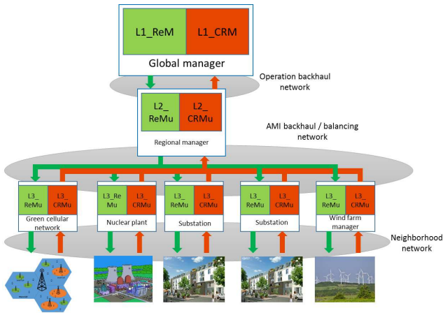
Figure 3. The HDCRAM architecture used as a management architecture for the global management of the electricity production and consumption
