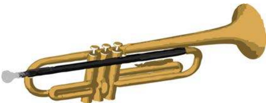
Fig. 2 Definition of the main parts of the trumpet: the mouthpiece (in light gray), the leadpipe (in black), and the flaring bell
