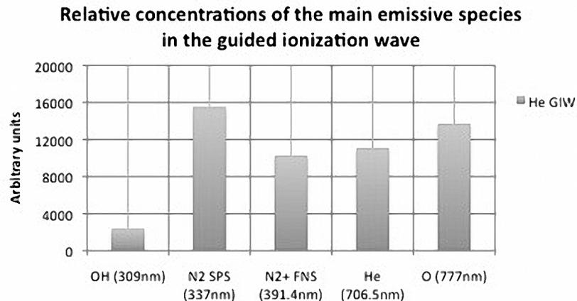
**Fig 3. Relative concentration of the main emissive species in the guided ionization wave (conditions: He gas flow = 2slm; voltage frequency = 10kHz; voltage amplitude = 5kV; voltage duty cycle = 1%. Optical fiber placed 5mm after the exit ceramic tube).**
