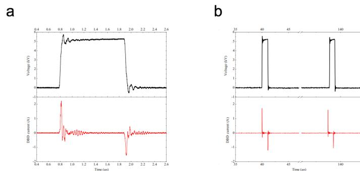
**Fig 2. Electrical high voltage and current signals analyzed during one impulse (2a) and during one period (2b) (He gas flow = 2slm, voltage frequency = 10kHz, voltage amplitude = 5kV, voltage duty cycle = 1).**
