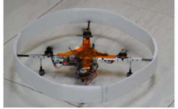
Fig. 1. Experimental aircraft equipped with the SBG and CHR sensor
