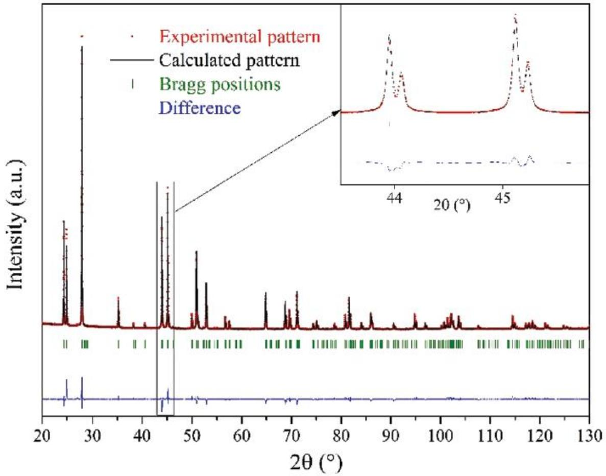
Fig. 4 Powder XRD Rietveld refinement of  $\text{Ce}_{0.975}\text{Sr}_{0.025}\text{F}_{2.975}$ .
