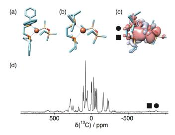
**Figure 2.** (a) X-ray structure of 1 (H atoms not shown for clarity). (b) DFT-optimized structure of 5. (c) Visualization of positive (blue) and negative (red) isosurfaces of spin density distribution in 5 (for  $\pm 0.0002$  a.u. isovalues). (d)  $^{13}C$  PNMR spectrum of 5. The two CH<sub>2</sub> carbons and their signals are labeled with a circle and a square in panels (c-d).
