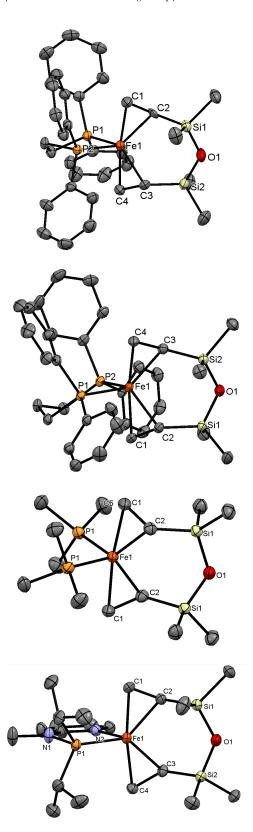
**Figure 1.** Thermal ellipsoid representation (at 50% probability) of complexes (from top to bottom) **1**, **2**, **3** and **4**; H atoms are not shown for clarity. Selected bond lengths (Å) and angles (°): For **1**: P1-Fe1-P2 84.75(3); P1-Fe1 2.302(10); P2-Fe1 2.316(10); C3-C4 1.419(5); C1-C2 1.409(5); for **2**: P1-Fe1-P2 91.37(2); P1-Fe1 2.291(6); P2-Fe1 2.335(6); C3-C4 1.418(3); C1-C2 1.415(3); for **3**: P1-Fe1-P1
