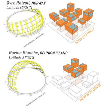
parametric modelling with dynamic solar simulation and evolutionary algorithm for solar urban planning. Thanks to their **flexibility**, it is possible to maximise the solar potential
