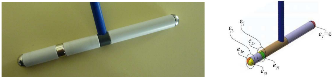
Figure 2. Photograph (left) and schematic view (right) of a 3-electrode sensor organized in 3 polarizable rings, 2 of them ( \mathcal{E}_2 and \mathcal{E}_3 ) being divided in two half rings ( e_{il}, e_{ir} ) allowing two lateral (left and right) current measurements.
