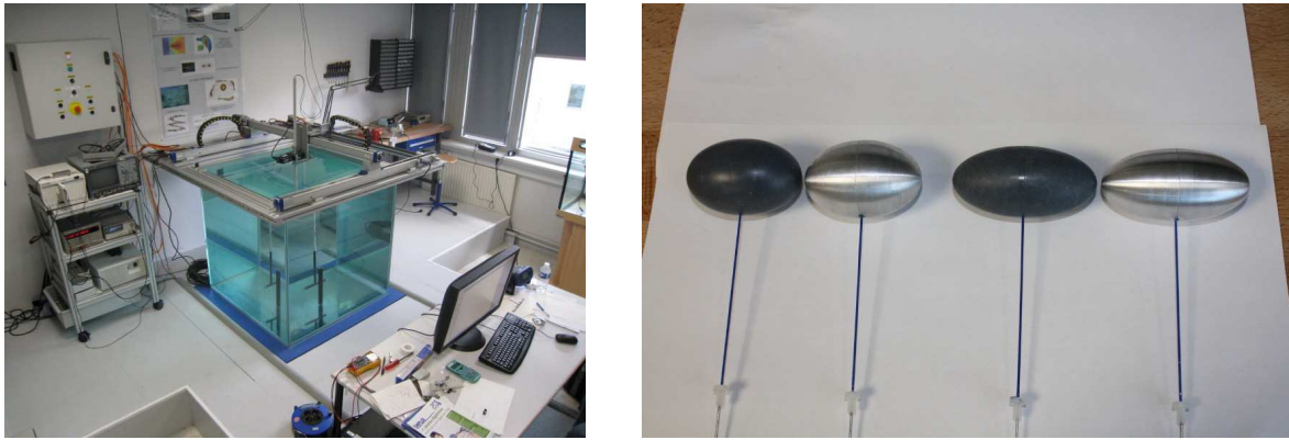
Figure 3. (left) Electrolocation test bench. (right) Example of a set of simple shaped objects (ellipsoids) of various sizes and materials (plastic, metal).
