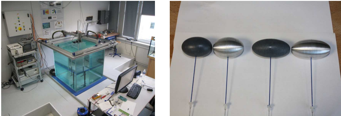
Figure 3. (left) Electrolocation test bench. (right) Example of a set of simple shaped objects (ellipsoids) of various sizes and materials (plastic, metal).
