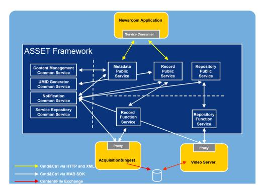
Figure 3 – ASSET demonstration platform components
