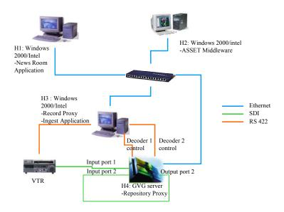
Figure 4 – ASSET network architecture for the demonstrator platform
