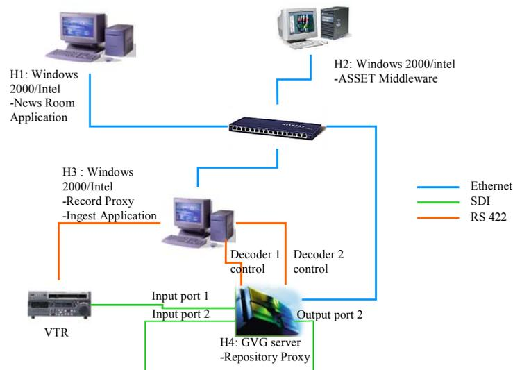
Figure 4 – ASSET network architecture for the demonstrator platform
