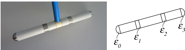
Fig. 3. Picture (left) and schematic view (right) of a 4-electrode sensor.
