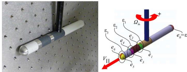
**Fig. 2.** Picture (left) and schematic view (right) of a 7-electrode sensor organized in 4 polarizable rings, 3 of them being divided in two half rings allowing two lateral (left and right) current measurements.
