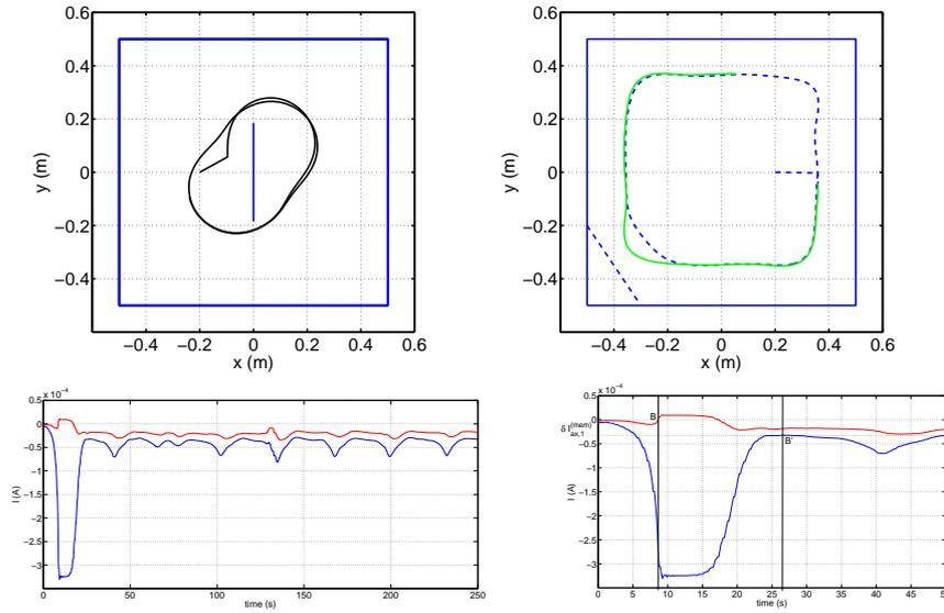
**Fig. 8.** (Top) Exploration of large objects. (Bottom) Time evolution of the currents  $\delta \bar{I}_{ax,1}$  (blue) and  $\delta \bar{I}_{ax,2}$  (red) along the sensor path when the sensor follows the tank walls.
