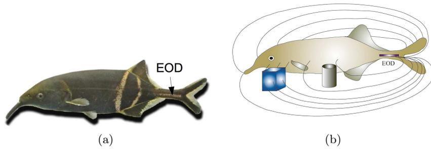
**Fig. 1.** (Left) The electric fish *Gnathonemus Petersii*. (Right) The electric field is distorted by the presence of an object (for instance, an insulating cylinder pushes the field lines away whereas a conductive cube funnels them).
