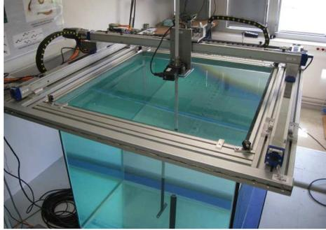
**Fig. 3.** Electrolocation test bench.
