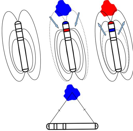
**Fig. 6.** (Top) The electric lines are pushed forward and backward depending if the object facing the sensor is conducting or insulating. (Bottom) When the head and tail electrodes are equidistant of the object, the head currents attain a minimum.
