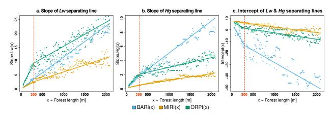
Figure 9: Influence of the length on the slopes and intercept of separating lines Hg and Lw and for a rock volume of 5 m<sup>3</sup>. The vertical dashed red line indicates the separation between short and long forest lengths.
