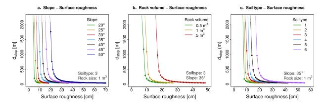
Figure 4: Distance from departure where 90% of the released blocks are stopped  $(d_{stop})$  in function of surface roughness (abscissa) and slope (a), rock volume (b) or soiltype (c).
