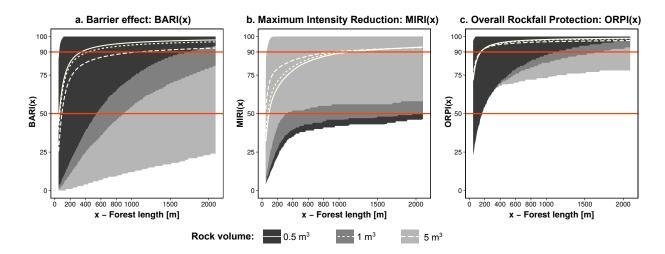
Figure 5: Effect of the forest length along the slope on the three indicators for the 3886 NFI plots. White lines show the average values for each rock volume. Gray-colored areas are placed on top of each other and represent the possible indicators values taken from the  $5^{th}$  percentile to the 95<sup>th</sup> percentile for each rock volume. Red lines represent the separating lines *Lw* (50) and *Hg* (90) between the three levels of protection used in this study.
