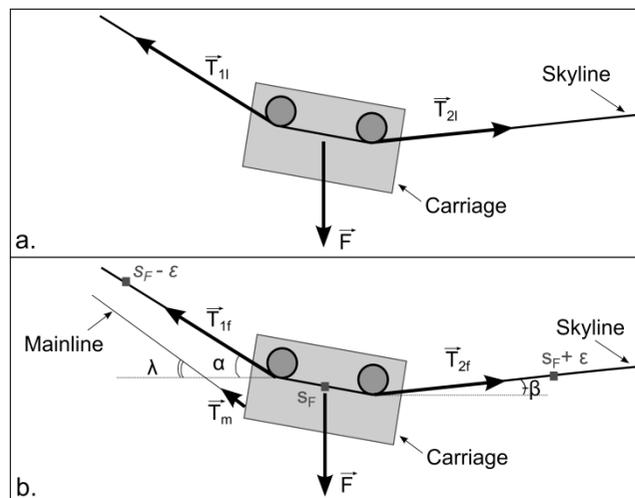
*Fig. 2 Forces acting in the equilibrium equation of the carriage. When the carriage is locked on the skyline or is self-motorized (a) the magnitude of the skyline tension at the upper side of the carriage  $T_{11}$  is greater than magnitude at the lower side of the carriage  $T_{21}$ . When the carriage is hold by the mainline (b) at curvilinear abscissa  $s_F$ , the magnitudes of the skyline tension at both sides of the carriage are considered as equal ( $T_{1f} = T_{2f}$ ).*
