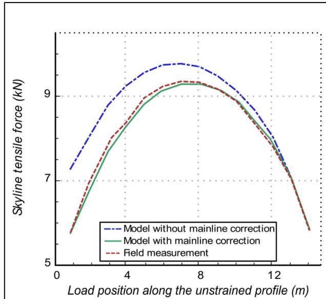
*Fig. 4 Comparison of skyline tensile force measured on field with the data predicted using the model with and without mainline tension correction for the configuration U2 - L. Corrected model prediction better fits the field measurement*
