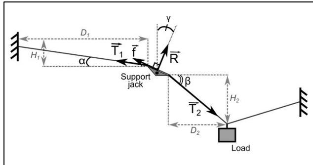
Fig. 3 Calculation of skyline friction at intermediate support
