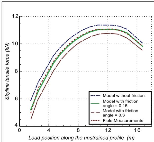
*Fig. 6 Influence of the friction of the skyline with the intermediate support on the skyline tension predicted by the model for the configuration Do2. If no friction is taken into account, the predicted tension is systematically above the measured tension. With a friction angle of 0.15 rad, experimental curve fits the modeling curve. Finally, with a friction angle of 0.3 rad, model predictions are above the experimental values*
