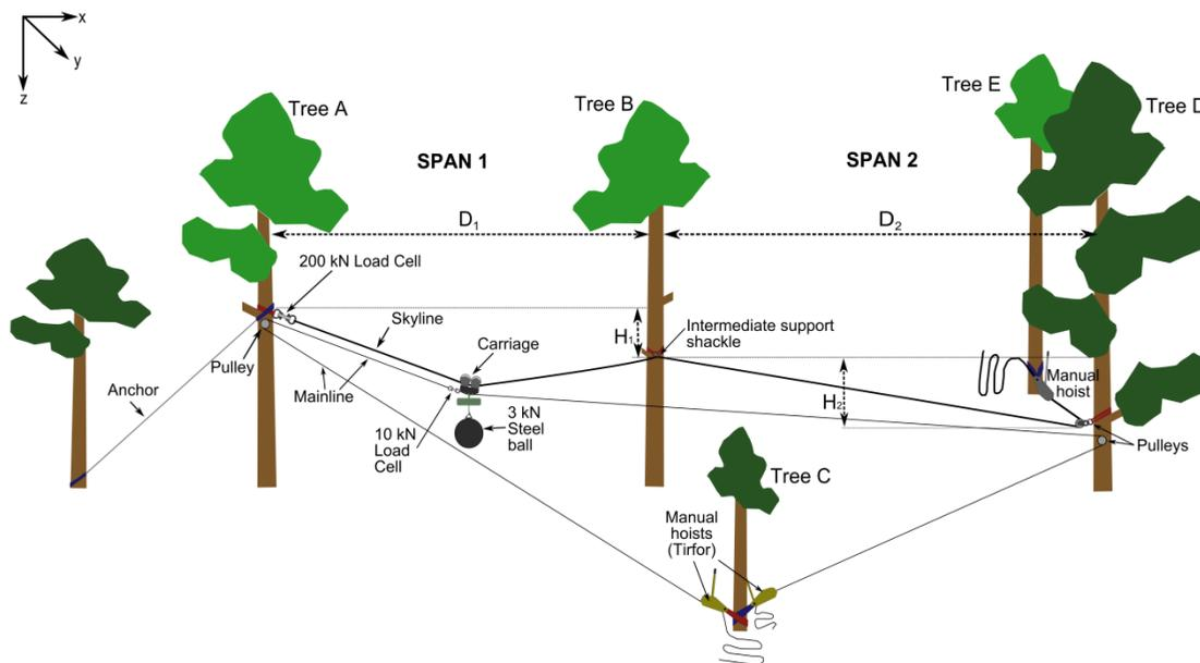
*Annex 3* Scheme of the real cable yarding operation followed. Measurements concern the situation when the load is located on SPAN 2 to ensure a full suspension of the log.
