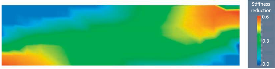
Fig. 6-13. Numerical stiffness reduction at the end of CEOS.fr RC wall 3 test.
