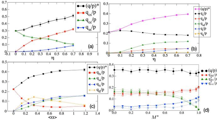
**Figure 5.** Normalized shear strength as a function of particle shape parameter or Mixing index, for (a)  $cs$ ,  $cc$  and  $ss$  contacts in packing composed of elongated particles, (b)  $s$ ,  $d$ ,  $sd$ ,  $t$  and  $q$  contacts in packing composed of non-convex particles, (c)  $ff$ ,  $fv$ ,  $fe$  and  $ee$  in packing composed of non-convex particles, and (d),  $dd$ ,  $dr$  and  $rr$  contacts for mixture of two shapes composed by the same proportion of disk and rcr.
