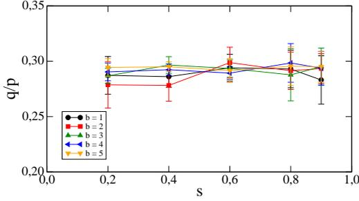
**Figure 3.** Shear strength  $(q/p)^*$  in the steady state as function of  $s$ , for all values of  $b$ .
