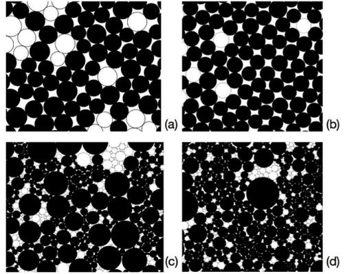
**Figure 2.** Zoom for  $(s = 0.2, b = 1)$ (a),  $(s = 0.2, b = 5)$ (b),  $(s = 0.9, b = 1)$ (c) and  $(s = 0.9, b = 5)$ (d) at the end of the isotropic compression. Floating particles (i.e., particles with one or no contacts) are shown in white.
