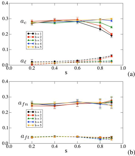
**Figure 5.** (a) Contact and branch length anisotropies,  $a_c$  and  $a_{ln}$  respectively, and (b) Normal and tangential force anisotropies,  $a_{fn}$  and  $a_{ft}$  respectively, all averaged in the steady state, as functions of  $s$ , for all values of  $b$ .
