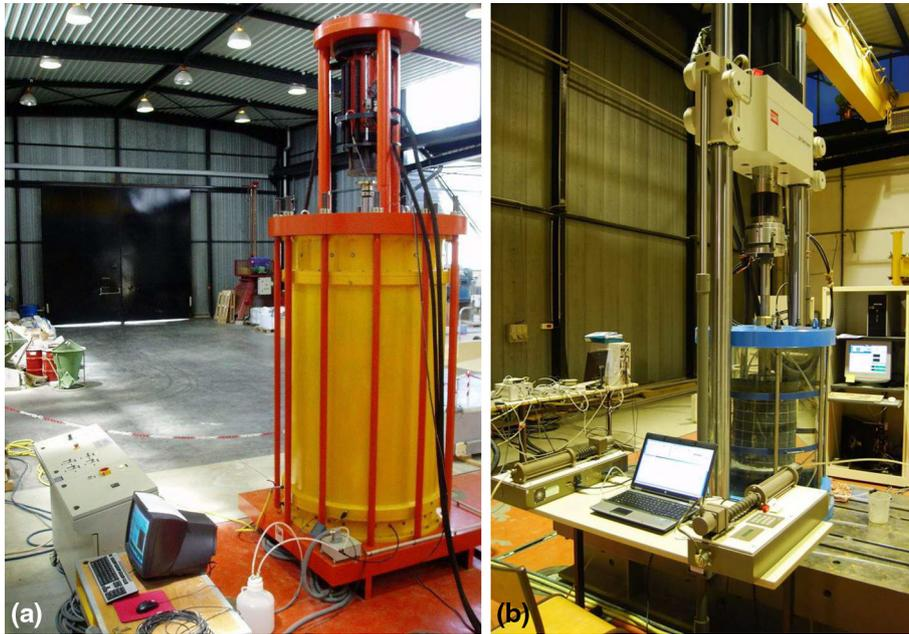
**Fig. 13** Large triaxial devices at the Ecole Centrale Nantes laboratory: **a** 1,000 mm diameter and 2,000 kN of max. vertical load; **b** 250 mm diameter and 500 kN of max. vertical load
