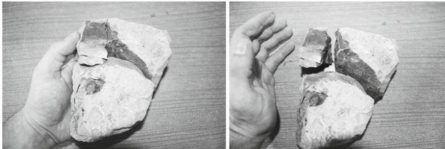
**Fig. 16** Coarse grain of STV crushed after a triaxial test
