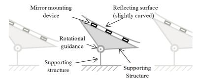
Figure 6 Schematization of solar collector
