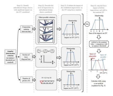
Figure 4 Illustrative example of ASR calculation procedure
