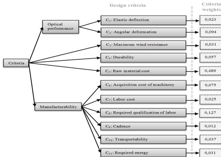
Figure 7 Design criteria with acceptance thresholds and weights
