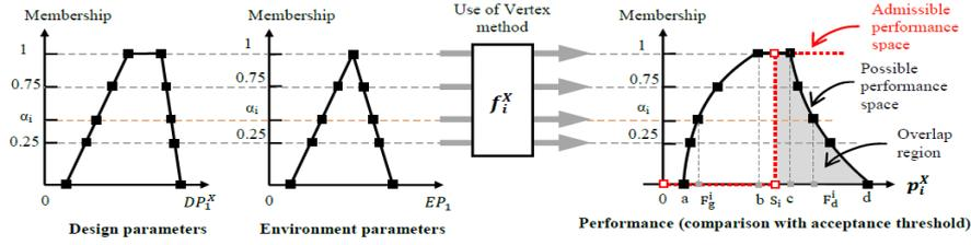
**Figure 5** Using the Vertex method to map design space to performance space (case of one design parameter and one environment parameter)
