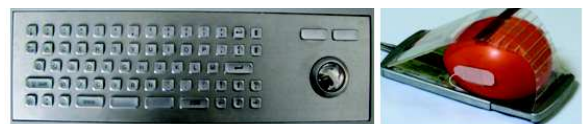
Figure 4: Illustration of the Human effectors property. Trackball keyboard [37]: \langle \text{keyboard: non dom. hand; trackball: dom. hand} \rangle (left). The Inflatable Mouse [22]: \langle \text{mouse: dom. hand; balloon: dom. hand} \rangle (right).
