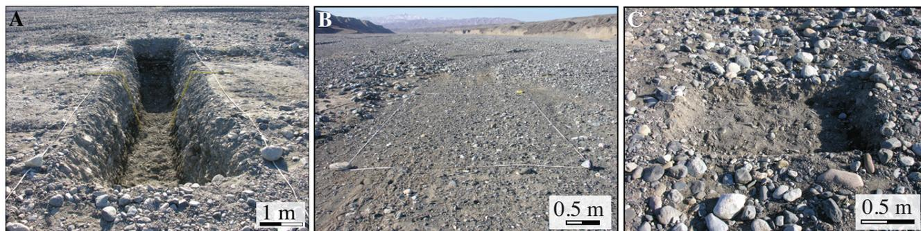
**Fig. 3.** (a) View of the deep trench dug to sample the Urumqi river bed. This trench is 7 m long, 1.2 m large and 0.8 m deep after removing the surface layer ( $\sim 20$  cm). (b) and (c) Examples of a grid and a shallow trench used to sample single morpho-sedimentary elements. The grid presented here is 4 m long and 3 m large, whereas the trench is 1.5 m long, 1 m large and 0.2 m deep.
