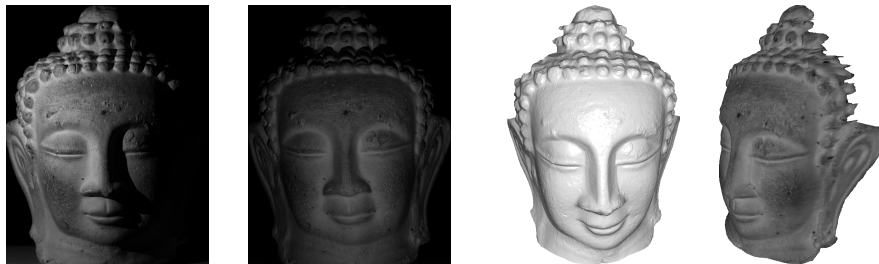
Fig. 1: Left: 2 out of m = 8 images of a plaster statuette. Each image is acquired while turning on one different nearby LED with calibrated position and orientation, but uncalibrated intensity. Right: result of our semi-calibrated PS approach, which automatically estimates the shape, the reflectance (mapped on the 3D-reconstruction on the rightmost figure) and the intensities.
