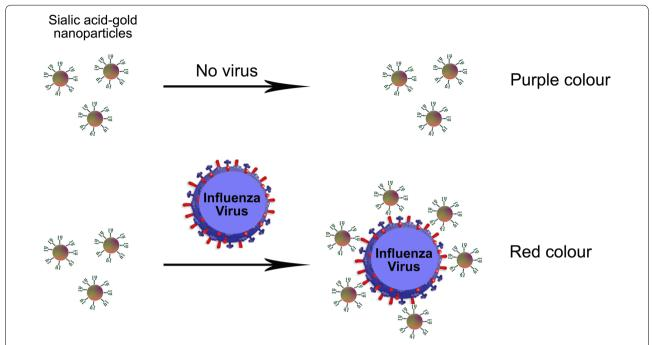
**Figure 2 Colorimetric sensor for detection of influenza A virus.** Sialic-mediated colorimetric detection of Influenza virus. Gold nanoparticles are stabilized with sialic to specifically bind HA protein on Influenza virus surface. Sialic-acid gold nanoparticles alone show the absorbance at 510 nm, while virus-bound nanoparticles absorbed at 600–610 nm. This allows label-free colorimetric readout for virus detection. Cartoon adapted from [42].
