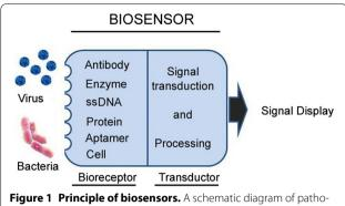
gen detection by a biosensor
