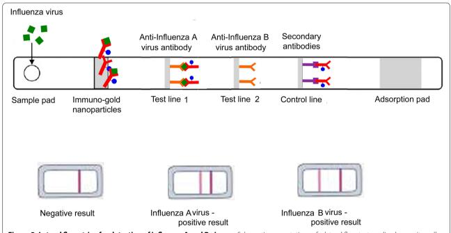
**Figure 3** Lateral flow strips for detection of influenza A and B viruses. Schematic presentations of a lateral flow tests realized on a nitrocellulose strips with immobilized antibodies against influenza virus A and B. A sample containing influenza virus flow by capillarity from the sample pad to bind test and control lines. In contrast, a sample without target virus flows from the sample application pad and binds only to the control line.
