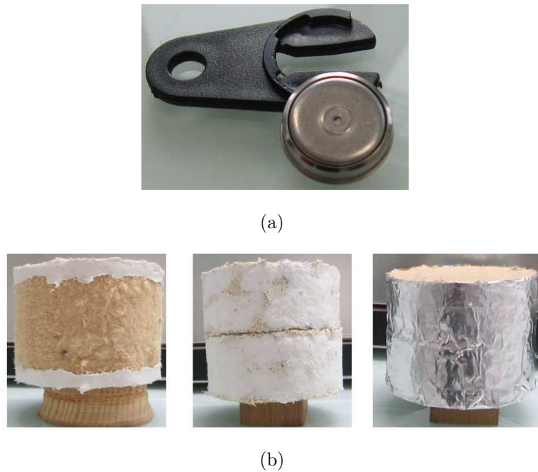
Figure 4. Sensors of relative humidity and temperature (a) and wood fibre samples (b) with white acrylic seal and with aluminium tape.
