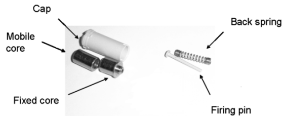
Figure 2. Components of electrical circuit breaker
