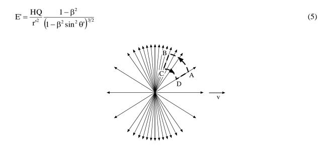
Fig. (2) Representation of the Field of a Uniformly Moving Charge
