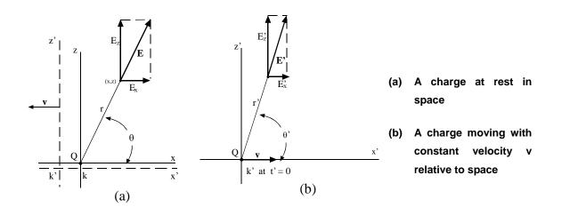
Fig. (1) The Electric Field of a Point Charge, Q
